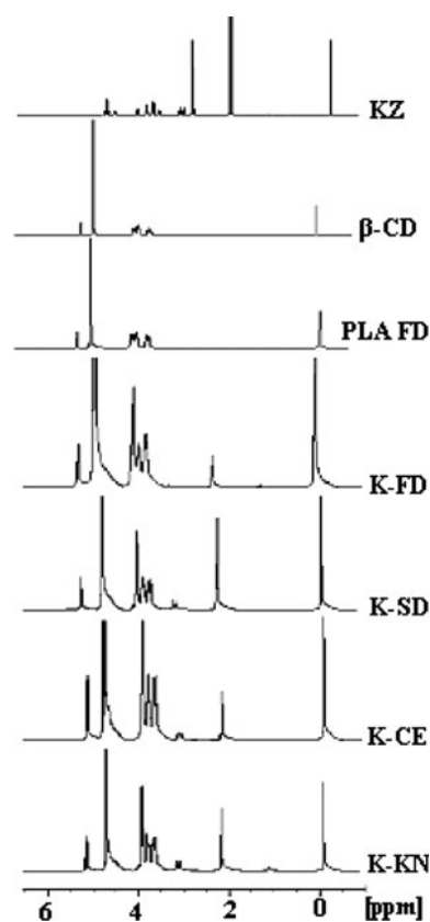
Fig. 5 ^1\text{H} NMR spectra of pure KZ, pure \beta -CD and KZ/ \beta -CD complexes
